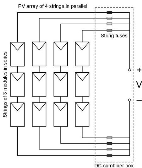
In this example there are 4 strings connected in parallel which all meet in the DC combiner box. Each string has 3 modules connected in series. For this example, the number 3 would have to be entered in the software under Modules and the number 4 under Strings.
